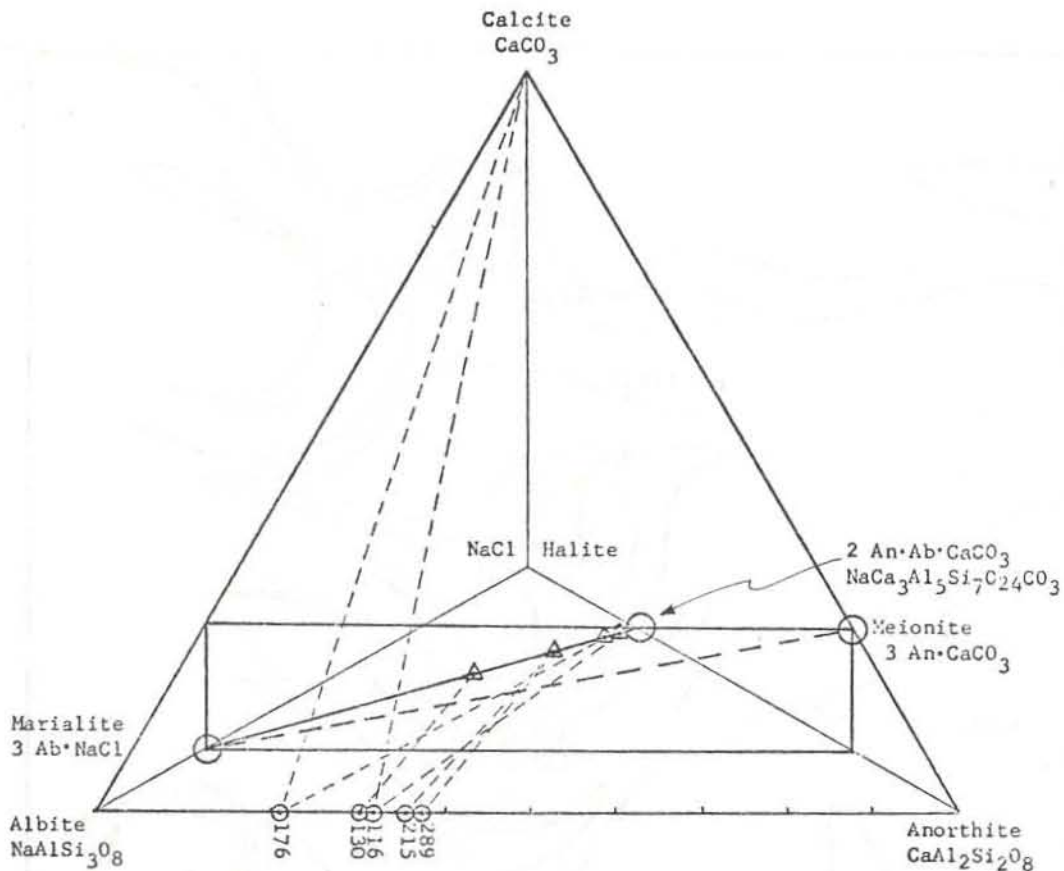
Figure 17. Composition tetrahedron albite-anorthite-halite-calcite. Scapolite composition plane 3 (albite + anorthite) : 1 (halite + calcite) is shown with solid line representing scapolite solid solution suggested by Evans and others (1969); dashed line represents previous stoichiometry. Plagioclase and scapolite compositions for analyzed samples are plotted.
