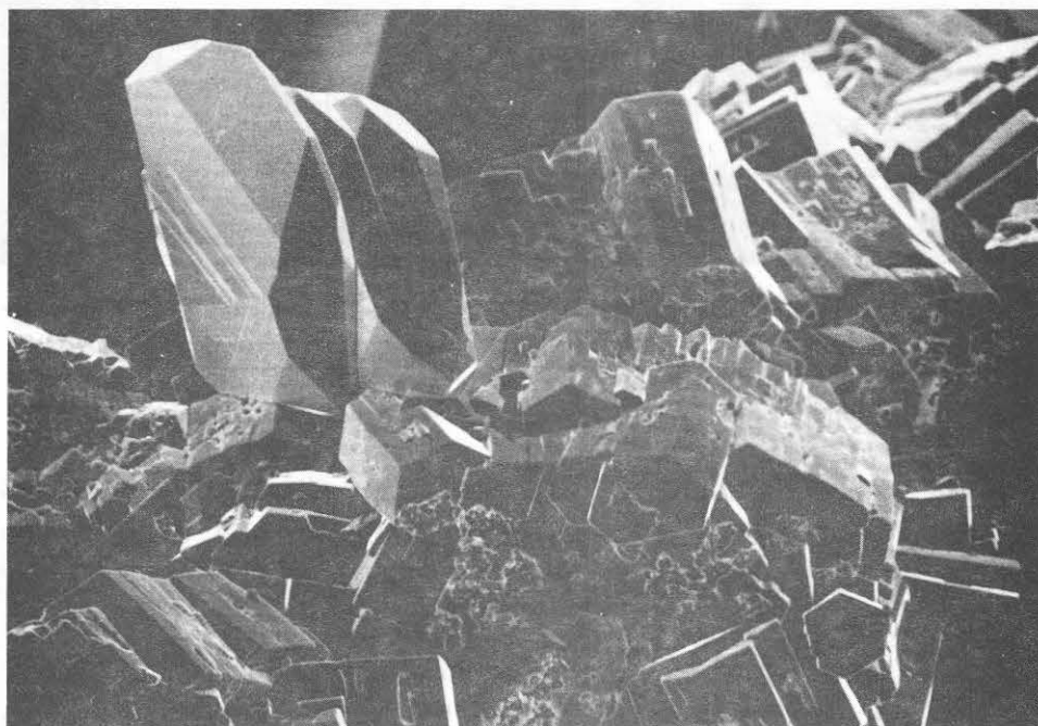
Figure 12. Black magnetite pseudomorphs after rhombohedral crystals of hematite with pink carbonate apatite crystals. The magnification of the SEM photomicrograph is about 200x. Photo by G. Robinson.
