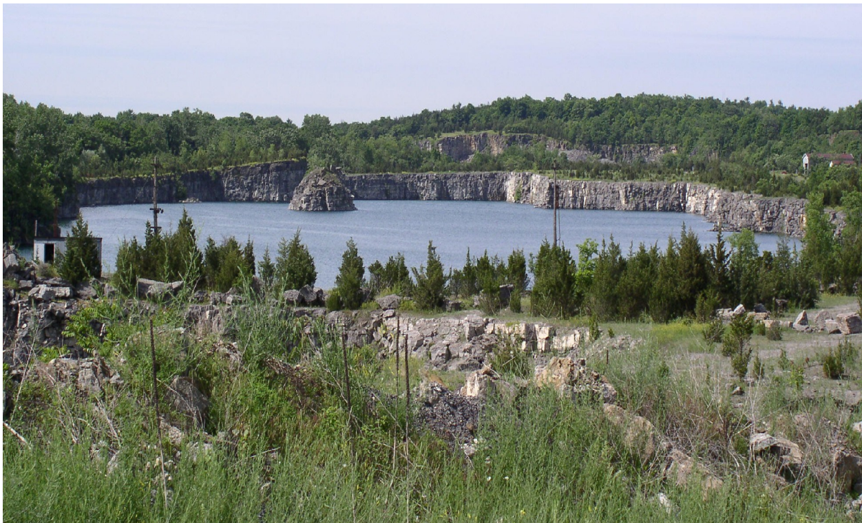
Figure 23. Photo showing water-filled (mine impoundment) at the Greenport Quarry. The excavated rock from the mined area in this photo was used largely for cement stone manufacturing.
