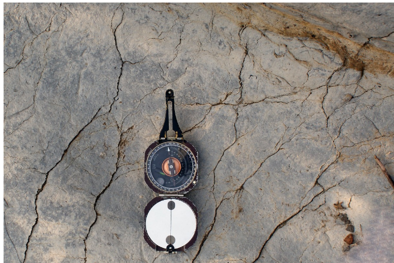
Figure 10. Photo of a bedding surface in the Onondaga Limestone, in north Kingston, illustrating two different cleavage orientations. The compass points due north. In the intersection orocline model, the earlier cleavage trends about N10°E, and the later cleavage dates about N30°E. The earlier cleavage is better developed, and may have continued to be an active locus of pressure solution even after the second cleavage starts to form, thus explaining ambiguous cross-cutting relationships.
