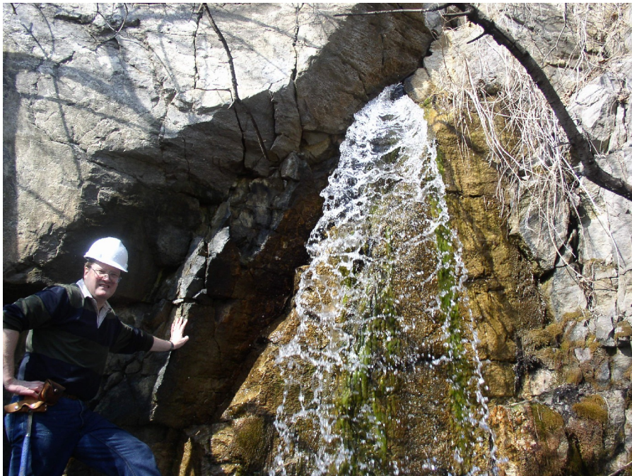
Figure 28. Photo of water-producing discontinuity in quarry wall. Flow is estimated at approximately 200 gpm.
