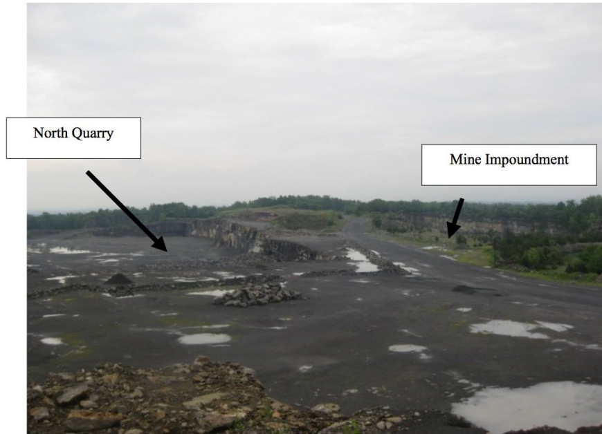
Figure 24. Photo showing differing elevations of mine impoundment surface (260 feet asl) on right and dry North Quarry floor (235 to 245 feet asl) on left.
