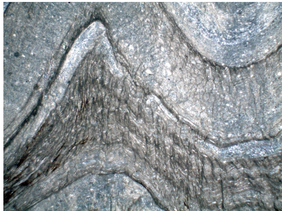
Figure 9. Thin section of kink fold and crenulation cleavage from Stop 2. The early foliation is bedding parallel and is folded by the later crenulation cleavage (vertical). The high phyllosilicate density in the crenulation cleavage domains suggests preferential dissolution of quartz. Field width 3.67 mm, PPL.
