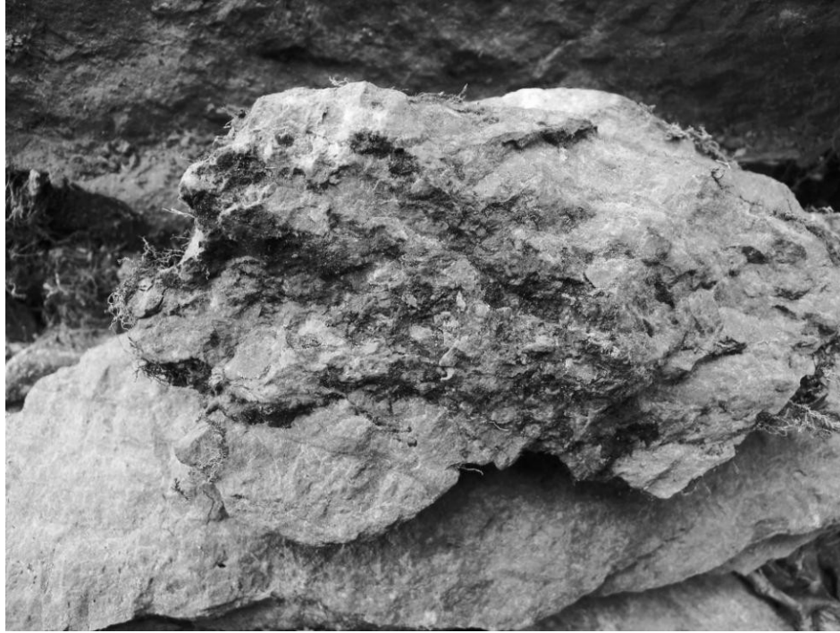
Figure 7. A closeup of the massive beds of Victor Dolostone at the lower Akron Falls. It takes a sledge hammer to examine the extremely resistant beds here. Stylonitic seams are common.
