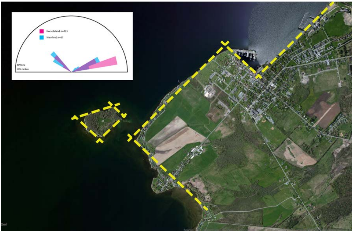
Figure 10. Satellite image of the Sackett's Harbour area highlighting the joint-controlled lakeshore and Horse Island (dashed lines). Inset is a rose diagram of both mainland and Horse Island joint data.
