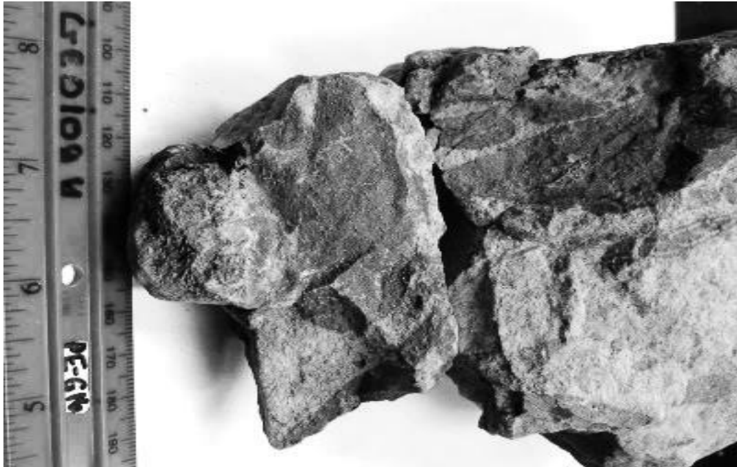
Figure 5. Explosion breccia sampled at the Schuyler mine consisting of diabase clasts in sandstone.
