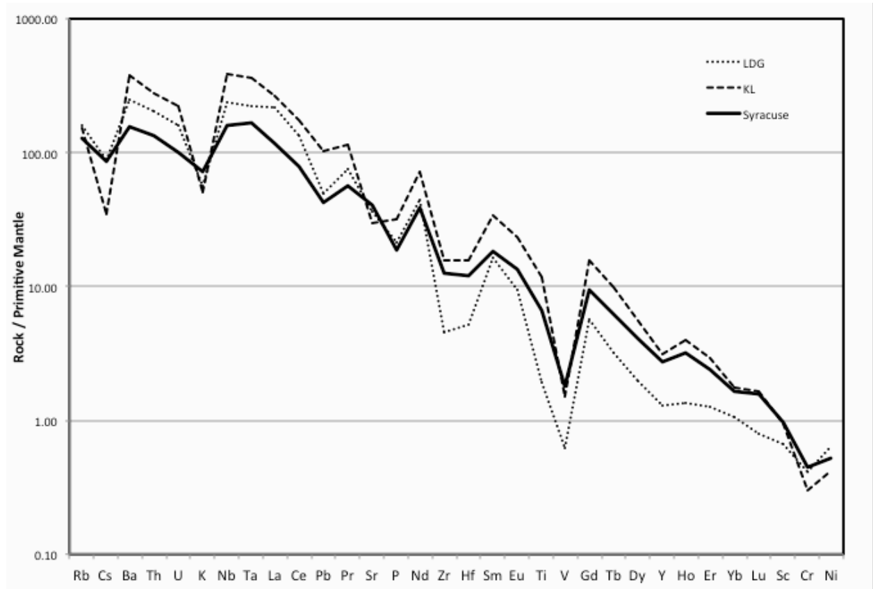
Figure 7. Primitive-mantle normalized spider diagram of trace element concentrations in the Syracuse kimberlites compared to the Lac de Gras (LDG) and Kirkland Lake (KL) kimberlites in Canada (average of six analyses of each). Data sources: Syracuse (Bailey, unpublished), Lac de Gras and Kirkland Lake (MacBride 2005) Normalizing factors from (McDonough and Sun 1995)
