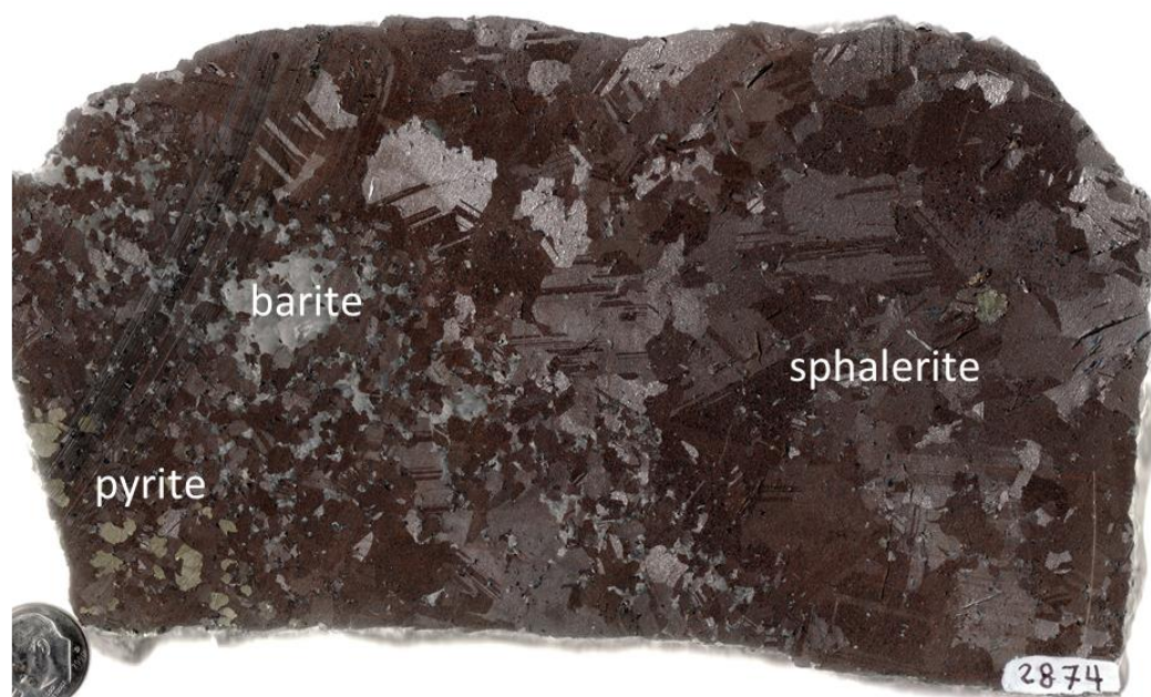
Figure 9. Coarsely crystalline sphalerite ore displaying interlocking twinned crystals, pyrite, and barite. Note the lack of brecciation and marble clasts typically found in ore associated with cross-cutting fault zones.
